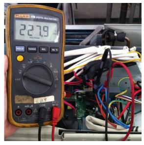
2 Turn off the power, use a digital tester to measure the resistance. The value should be  $1.8\sim2.5~\text{K}\Omega$ .
